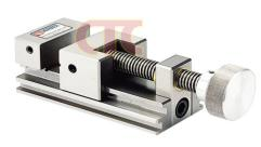
Material: SKS2 Hardness: HRC 58°-60° Squareness: Within 0.005m/m It was made by tool steel of stainless steel system and was precision ground after hardened by heat treatment. So, it will not be rusted even though permeation.
